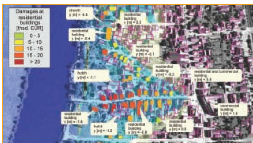
Fig. 4.3: A local GIS-based flood risk map showing the economic damage for a flood that occurred in 1993 in Offenau in Neckar, Germany (Del.2.1.1.1-B.I-37) Original Source: Buchlel et al. (2006)
